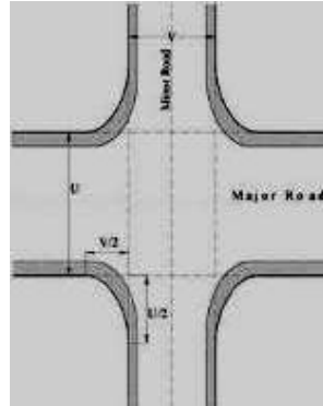
Figure 2: Rounding off intersection of roads meeting at 90 degrees →
